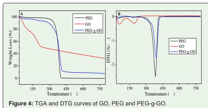
Figure 4: TGA and DTG curves of GO, PEG and PEG-g-GO.
