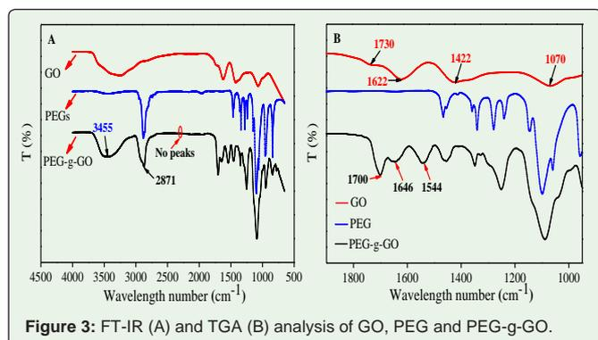
Figure 3: FT-IR (A) and TGA (B) analysis of GO, PEG and PEG-g-GO.
