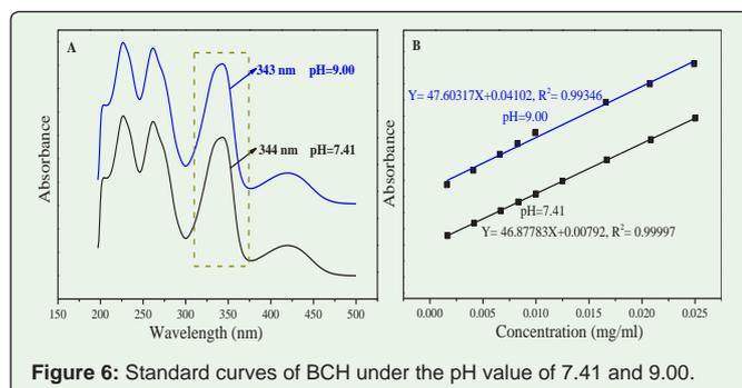
Figure 6: Standard curves of BCH under the pH value of 7.41 and 9.00.
