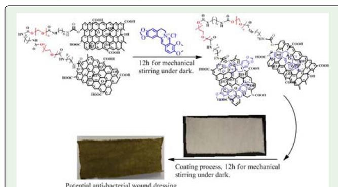
Figure 2: The process of BCH loading on PEG-g-GO carrier, and the subsequent coating on cotton fabric.
