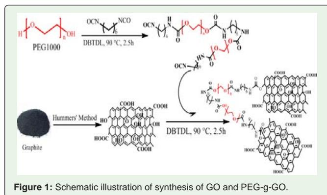
Figure 1: Schematic illustration of synthesis of GO and PEG-g-GO.
