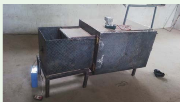
Figure 2: Plate 1- Pneumatic kiln [3].
