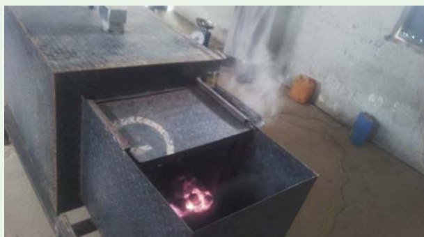
Figure 3: Plate 2- Pneumatic charcoal kiln showing the charcoal, smoking and fan chambers.
