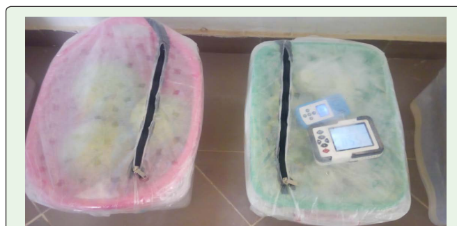
Figure 1: The setup of HMAS with oxygen and carbon dioxide readers enclosed during periodic Reading.
