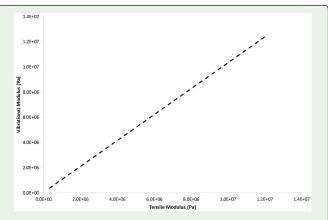
**Figure 2:** Calibration curve of modulus determined from vibrational studies and conventional tensile testing. This plot shows the modulus determined from a combination of vibrational stimulation and OCT is directly related to the modulus measured in a tensile incremental stress-strain test as reported previously [40-42].
